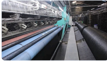
Proses tenun benang HDPE + stabilizer UV
